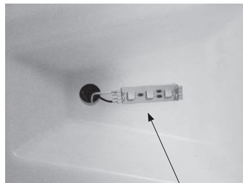
Peel LED PCB (DB-60030UK) away from inner disc
